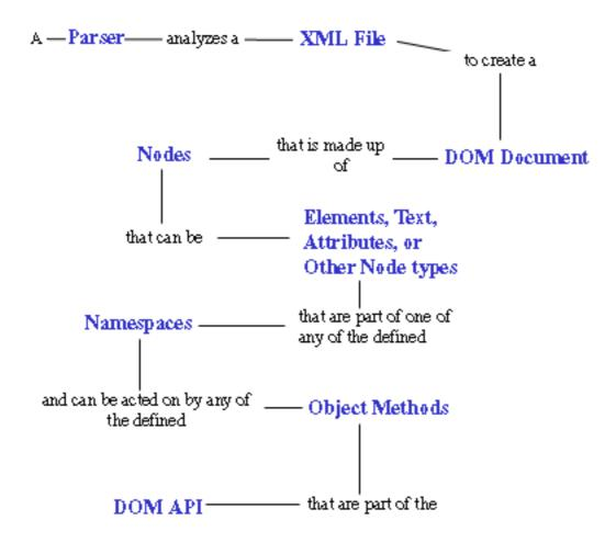
A **parser** is a software application that is designed to analyze a document -- in this case an XML file -- and do something specific with the information. In an event-based API like SAX, the parser sends events to a listener of some sort. In a tree-based API like DOM, the parser builds a data tree in memory.
