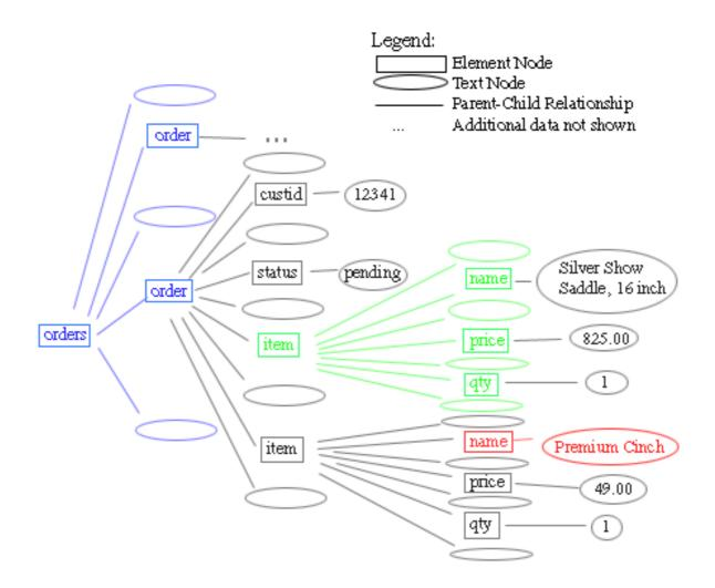
The rectangular boxes represent element nodes, and the ovals represent **text nodes**. When one node is contained within another node, it is considered to be a **child** of that node.
